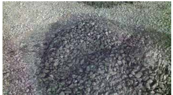
Fig. 8: The first concrete out of the chute is typically segregated toward the top-size aggregate
