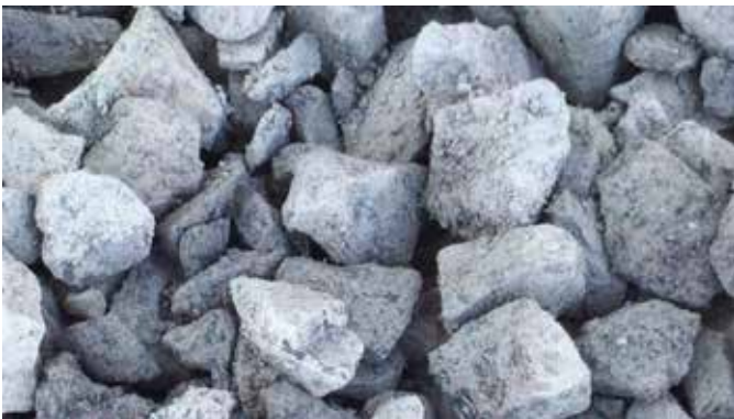
Fig. 9: Coarse aggregate particles coated with fine materials may interfere with bond and thus contribute to flaking
